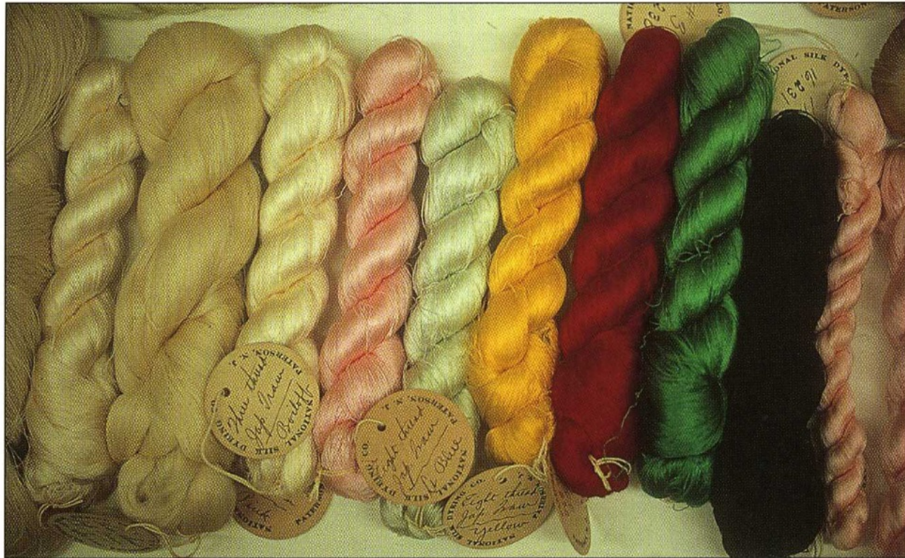
Skeins of weaving yarn made from Japanese raw silk. From left: lustrous bleached white; dull white still in the gum; white boiled off three thread tram; light pink and light blue eight thread tram; yellow eight thread tram; less lustrous red, green and black spun or schappe silk; lustrous pink tram. Courtesy The Collection of the Newark Museum. Gift of the National Silk Dyeing Company, Paterson, New Jersey, 1916.
